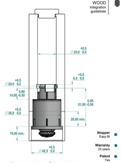
All measurements in mm. Tolerances shown are for mounting into wooden products. Minimum 6mm wall thickness around ribs recommended for wooden products.
